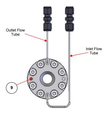
Fig 5. Front view of High Pressure Liquid Cell (without its slide mount backplate) showing thermocouple connection point (9) when cell is installed in the Electrical Heating Jacket
