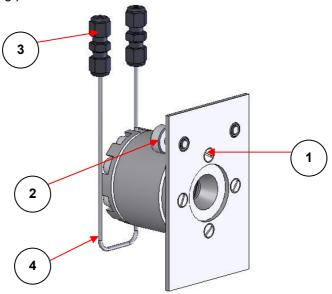
Fig 2. Fitting of the 3" x 2" slide mount backplate to the High Pressure Liquid Cell
