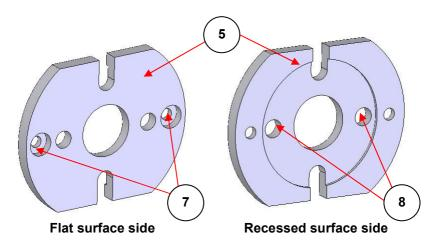
Fig 3. Front cover plate (both sides seen) to hold High Pressure Liquid Cell when placed in the Electrical Heating Jacket GS20730
